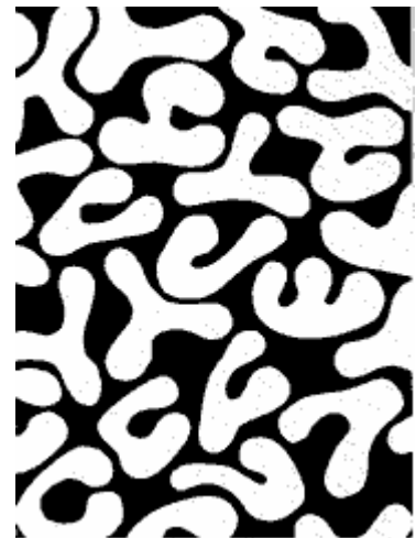
The highly profiled P84 fibers cover a large surface area. Dust collection occurs on the surface of this media and will not easily blind.
